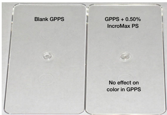
2. Visual aspects of molded GPPS plaques containing no IncroMax PS and 0.50% IncroMax PS for color comparison
