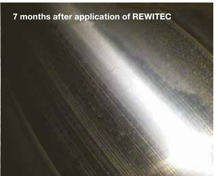
Figure 16 Surface grooves at planetary bearing before and after the application of REWITEC
