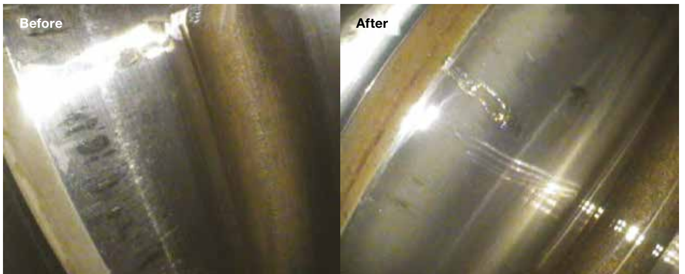
Figure 20 Sun pinion wear, before and after the application of REWITEC
