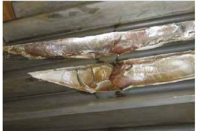
Figure 2 Overload breakage on a tooth flank
