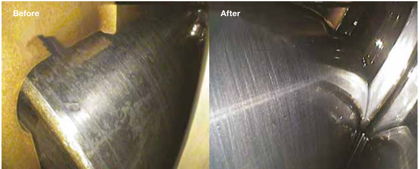
Figure 19 Micropitting on a bearing element before and after the application of REWITEC
