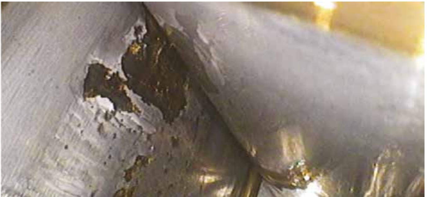
Figure 13 Spalling on a bearing
