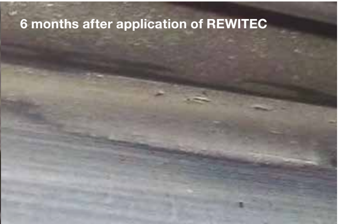
Figure 15 Micropitting after the REWITEC application
