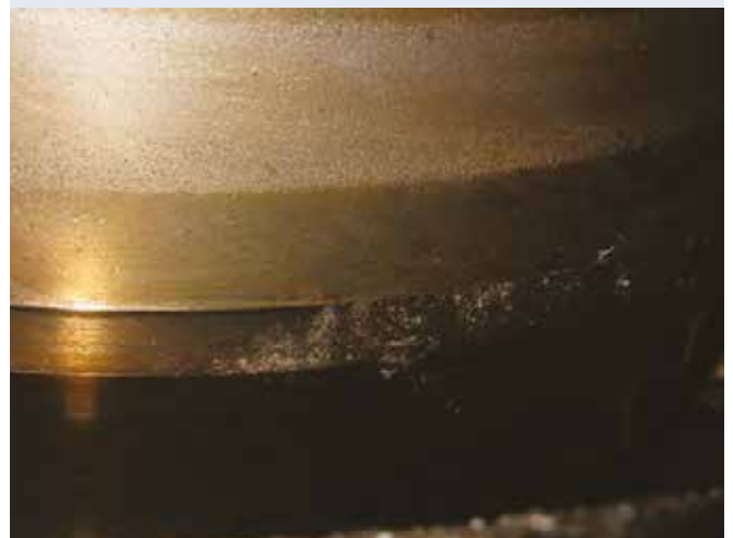
Figure 9 Surface fatigue phenomena on a bearing ring
