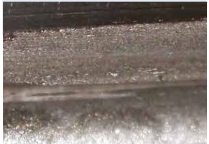
Figure 7 Tooth flank with micropitting and corrosion
