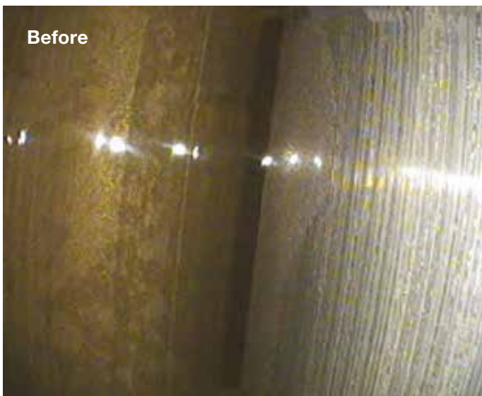
Figure 16 Surface grooves at planetary bearing before and after the application of REWITEC
