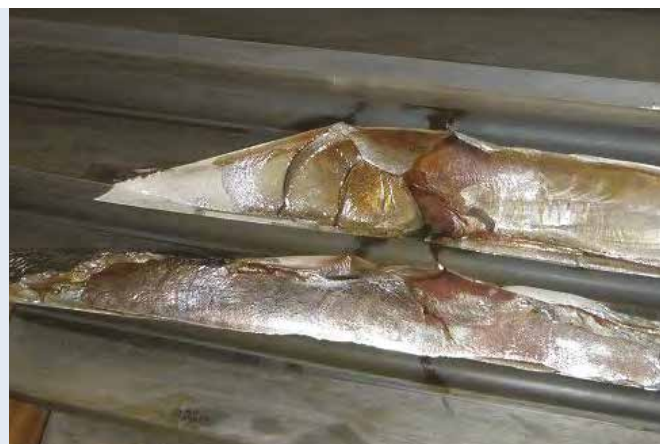
Figure 3 Overload breakage on a tooth flank
