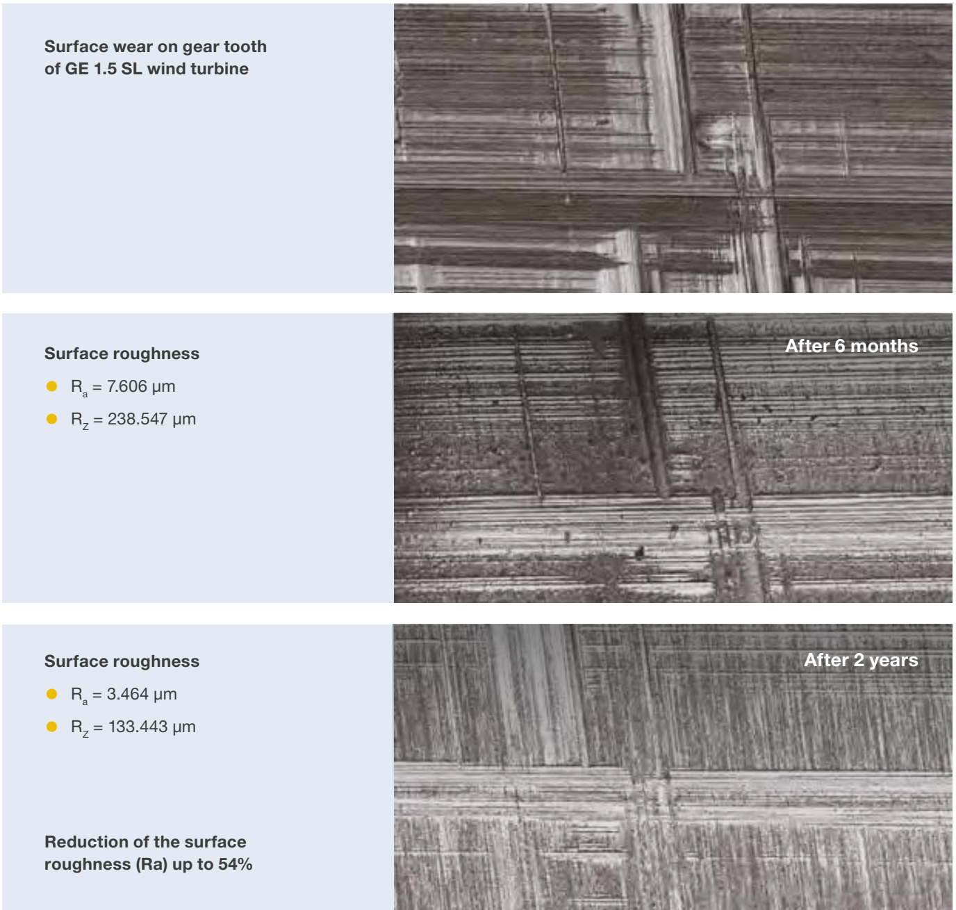
Figure 22 Surface roughness evaluations before and after the application of REWITEC
