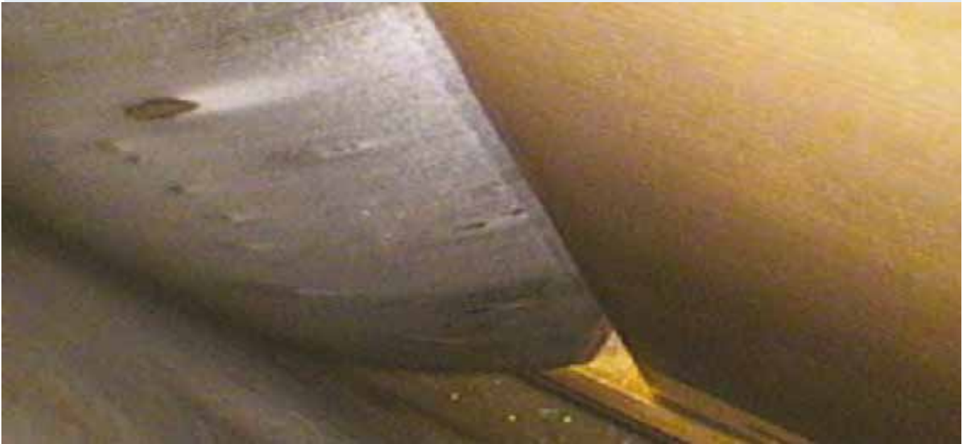
Figure 12 Spalling on a bearing
