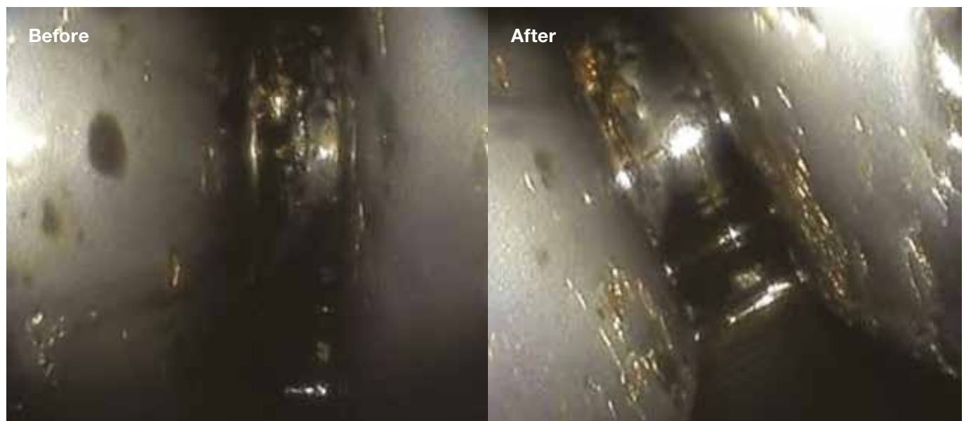
Figure 18 Rolling element in a planetary bearing, before and after the application of REWITEC
